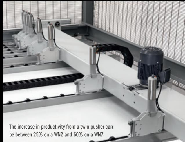
The increase in productivity from a twin pusher can be between 25% on a WN2 and 60% on a WN7.
