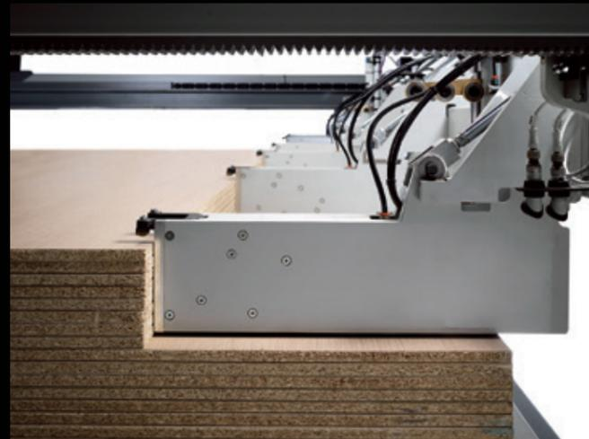
of the machine, even if the frame moves slightly, the saw carriage will remain parallel to it. No one else in the market does this.
